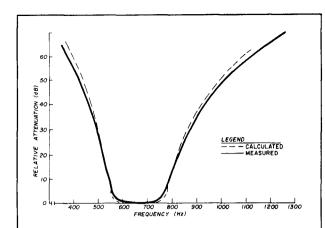
fig. 3. Measured and calculated attenuation responses of the CW filter in fig. 2. The measured response differs slightly from the calculated response because the resistive losses of the filter were not included in the calculations.
